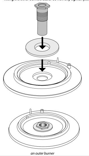
When all the burner bases and venturis have been fitted tighten the venturi nuts.
